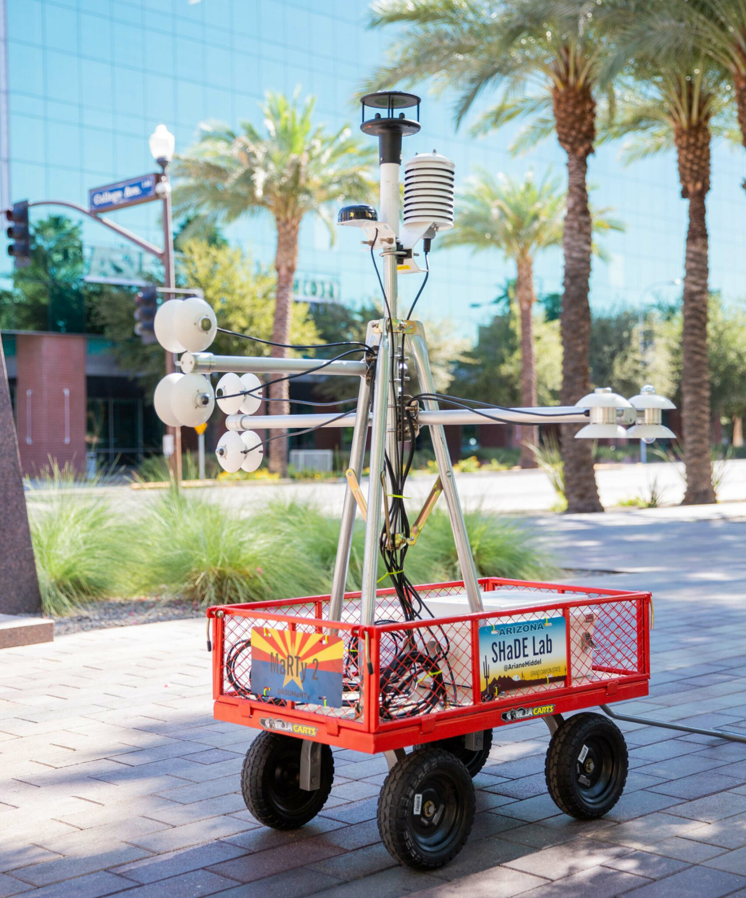
MaRTy is a "mobile biometeorological instrument platform that measures air temperature, humidity, wind speed and direction, GPS coordinates, and MRT (Mean Radiant Temperature) using the 6-directional method." Photo courtesy of SHaDE Lab, Arizona State University.
