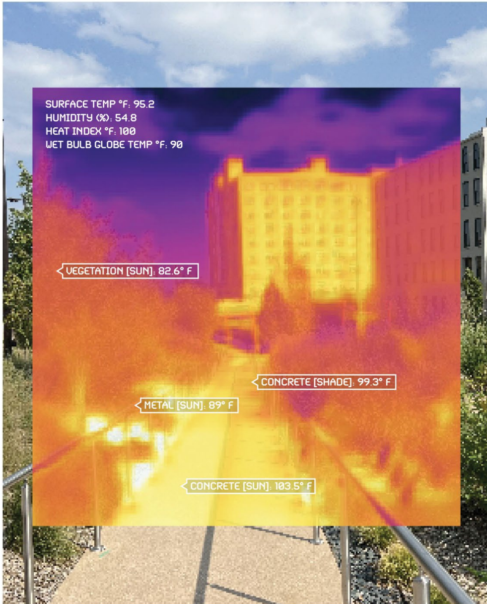
Handheld thermal image of an ADA ramp at the Gene Leahy Mall.
