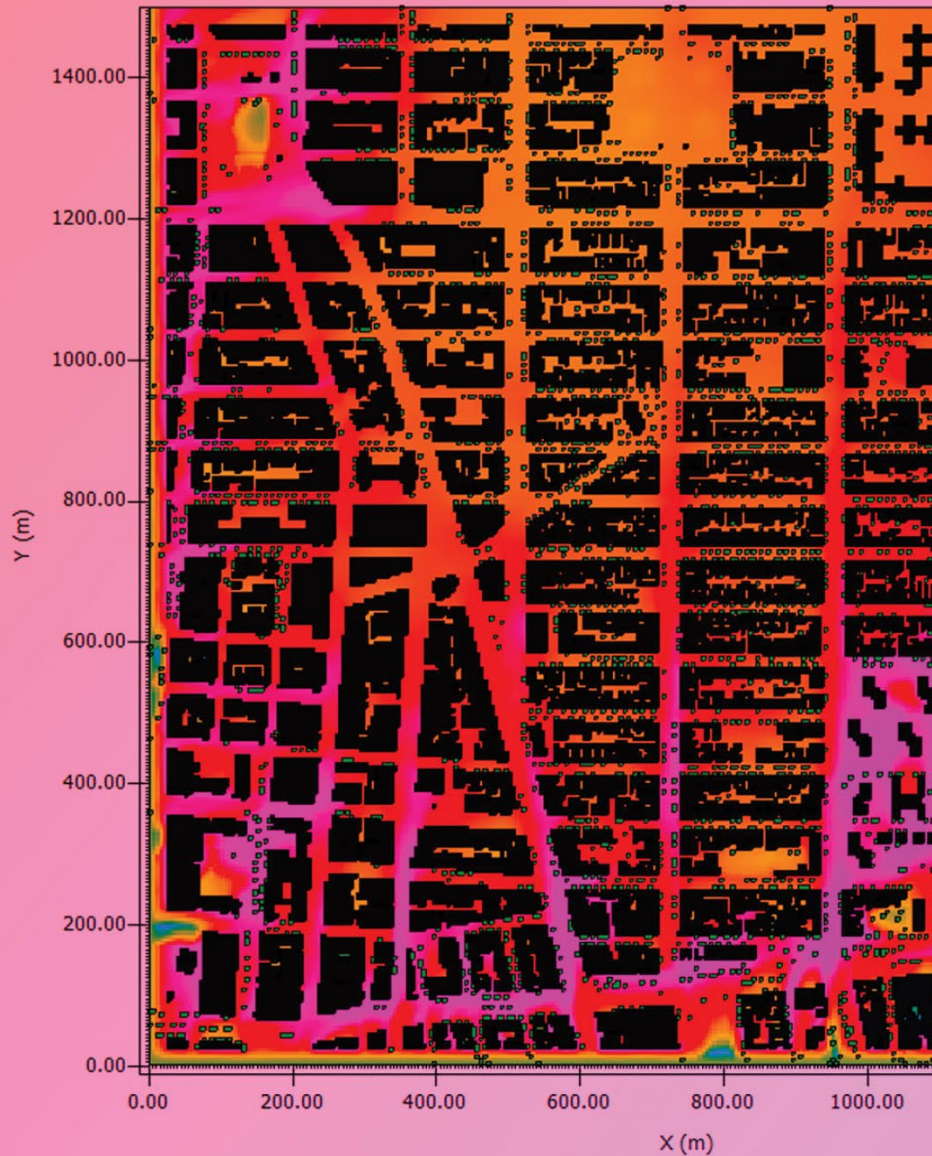
Sample of urban heat island mapping using ENVI-met, an environmental simulation software. 1
